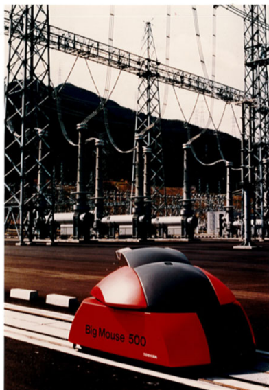
A ROBOT TO PATROL SUBSTATION (PATROL ON THE GROUND)
